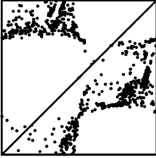
FIG. 4. Map for angles of return times for the periodically forced Rössler system in a chaotic regime. The parameter values are given in the text.
